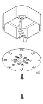
Note - Make sure the supplied Universal Mounting Plate is fastened directly to the junction box. The surface of the junction box should be set back 1/8" or 3mm from the mounting surface. This will ensure the best possible fit for ease of installation and final finish. Note below the correct and incorrect fit for optimum installation.
